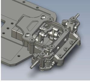
5. Install servo post onto servo using provided \*\*\* screws(\*Flat side facing servo)\*Note: Servo Horn Not Included
