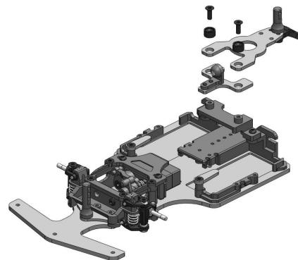
8. Place battery holder ring in between the chassis and the rear base, make sure it's placed around the screw hole then install the provided screws from bottom of the chassis to secure the rings.
