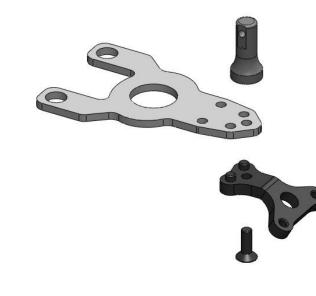
7. Prepare the damper with body post and wing mount, use M2x8 screw from bottom to top
