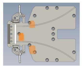
3. Secure front suspension assembly onto chassis using provided \*\*\* screws
