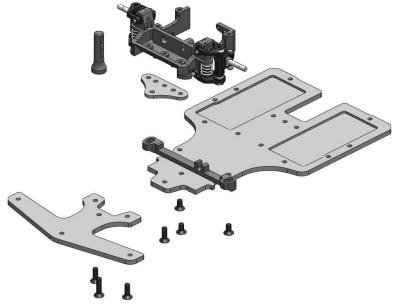
2. Insert tie rod into the slot and sandwich it between front suspension assembly and the chassis.
