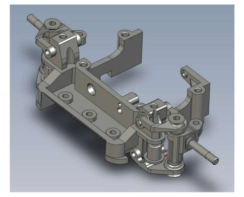
1. Install double a arm components onto front bulkhead.
