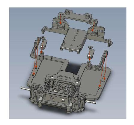
8. Place battery holder ring in between the chassis and the rear base, make sure it's placed around the screw hole then install the provided screws from bottom of the chassis to secure the rings.
