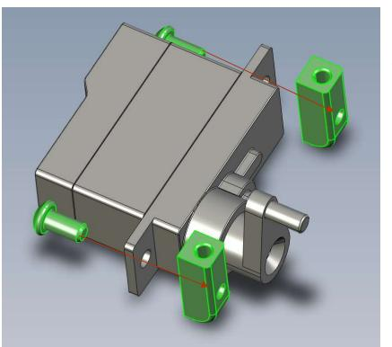
5. Install servo post onto servo using provided \*\*\* screws (\*Flat side facing servo)
