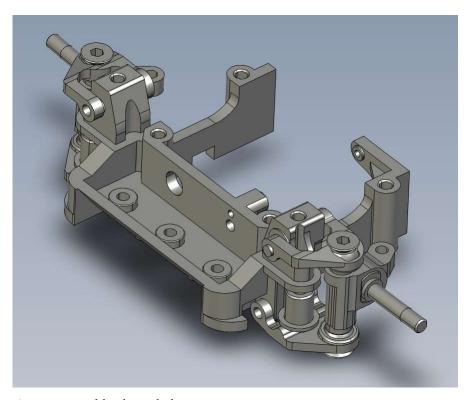
1. Install double a arm components onto front bulkhead.
