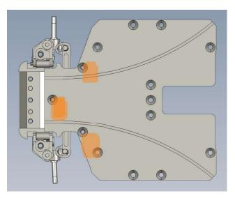
3. Secure front suspension assembly onto chassis using provided \*\*\* screws
