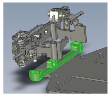
2. Insert tie rod into the slot and sandwich it between front suspension assembly and the chassis.
